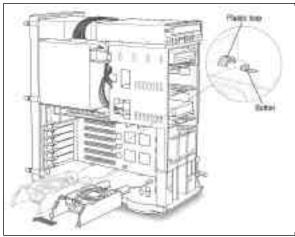
Reinstalling the fan (retaining clip on 8500)
